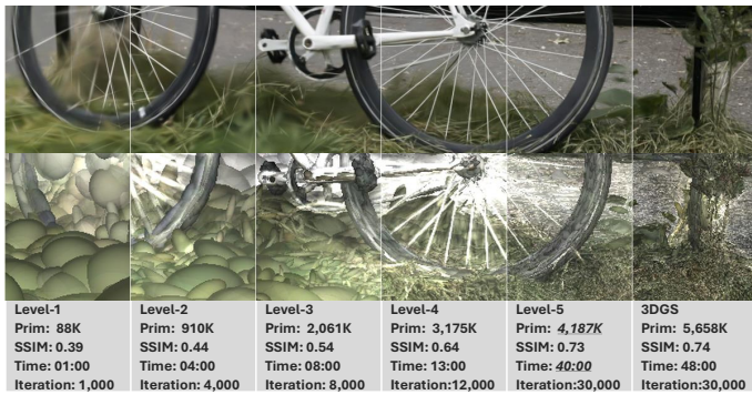
Figure 1: Top: RGB rendering. Middle: Gaussian Visualization. Bottom: Size, SSIM, cumulative training time and global iteration. Each column indicates one level of detail used in our coarse-to-fine optimization and the last column shows 3DGS for comparison.
